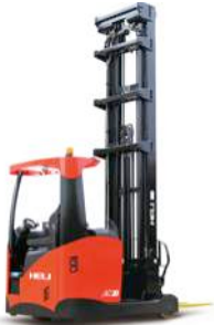
Reach Truck- Battery 1 – 2 tons Up to 12.5m
