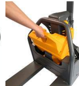
1 Minute replacement Lithium Battery
